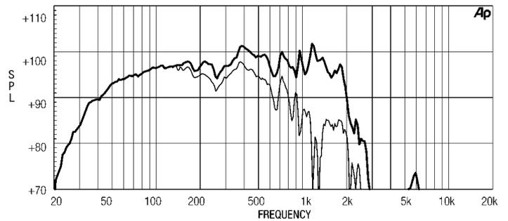
**FREQUENCY RESPONSE CURVE OF 21LW1400 MADE ON 250 LIT. ENCLOSURE TUNED 28HZ IN FREE FIELD (4PI) ENVIRONMENT. ENCLOSURE CLOSES THE REAR OF THE DRIVER. THE THIN LINE REPRESENTS 45 DEG. OFF AXIS FREQUENCY RESPONSE**
